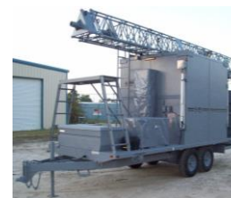
Mobile Cell Tower
